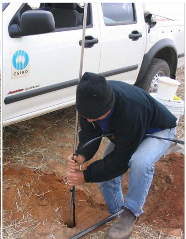
**Figure 2.3** Pushing the drainage meter into the 92 mm diameter borehole.
