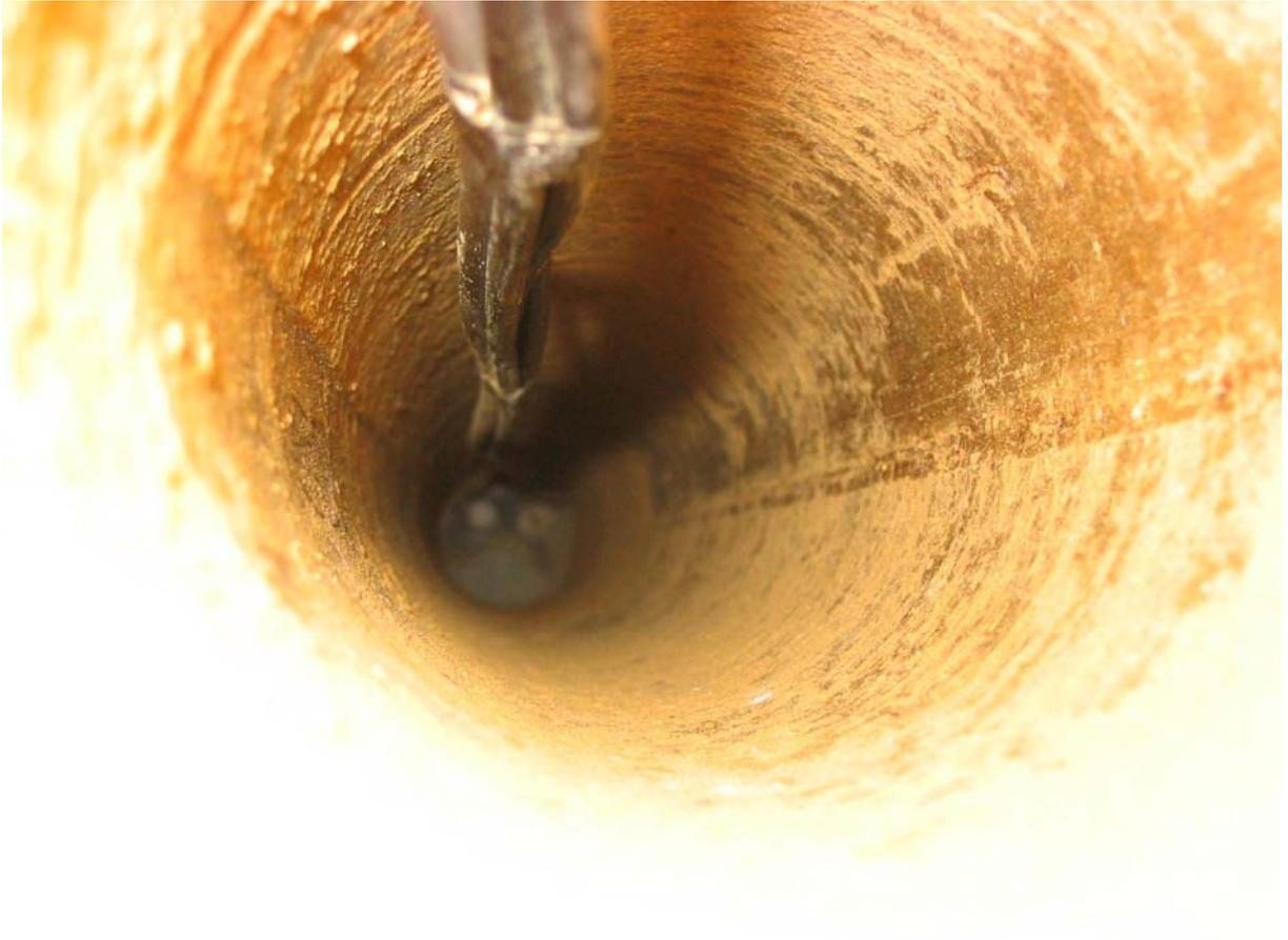
**Figure 2.5** View down the installation borehole after packing the lower tensiometer sensing tip. The top of the upper tensiometer tube and the scintered glass plate for solution injection/withdrawal can be seen next to packed bentonite above the lower tensiometer.
