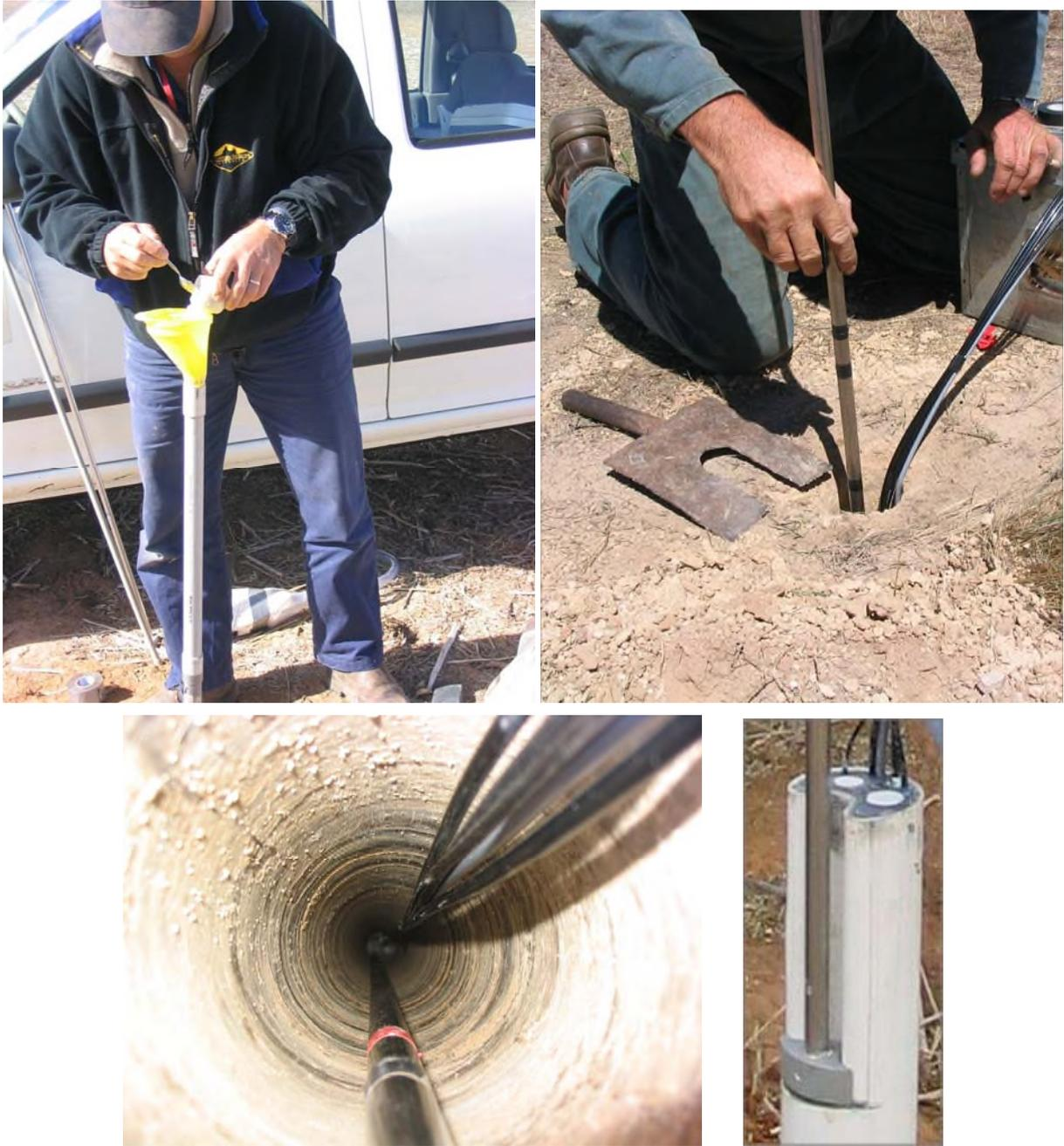
**Figure 2.4** Packing diatomaceous earth to form the lower tensiometer sensing tip. Note the specially shaped packing tool (bottom right)
