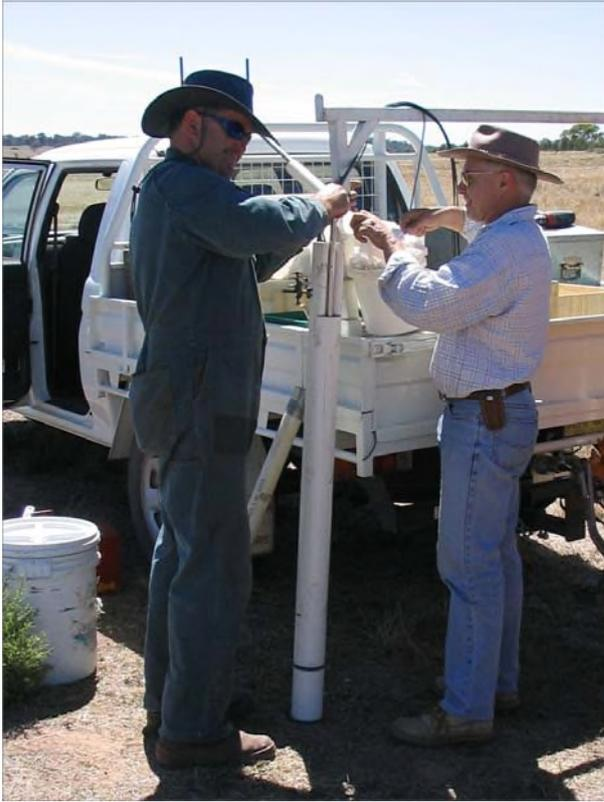
**Figure 2.1** Packing the tube tensiometers with diatomaceous earth prior to installation
