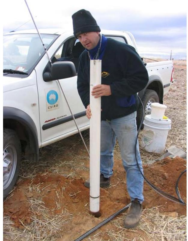
**Figure 2.2** Preparing to insert the drainage meter into the 92 mm borehole.
