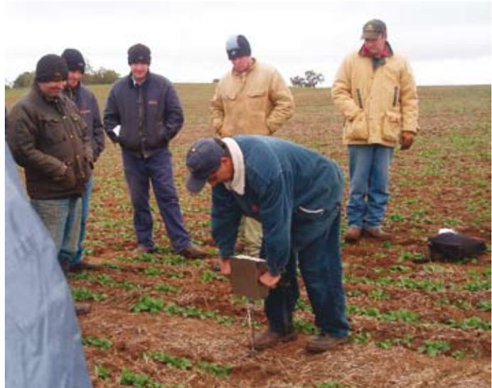
Measuring soil strength using a penetrometer at the Bobbara Station Field Day 2007.
