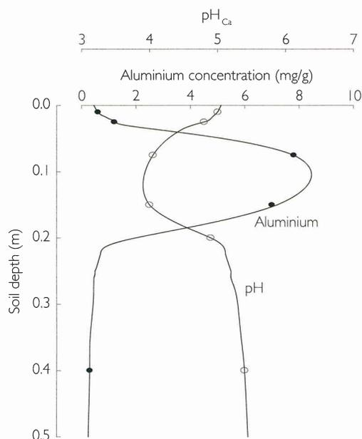
> Figure 1. Example of the profiles of pH and aluminium concentration in a Harden soil with an acid throttle.
