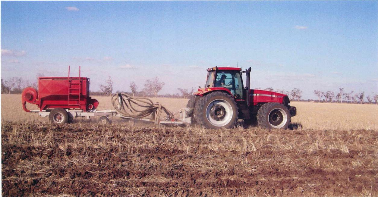
> Figure 3. Implement that injects dry lime into the subsurface behind ripper tines (courtesy of Farmlink and Yeomans Plow).
